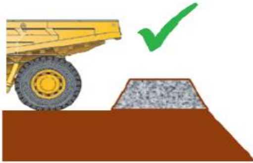
SUITABLE EDGE PROTECTION BERM PROFILE
