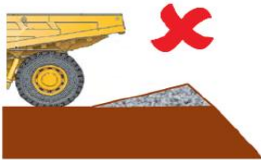
UNSUITABLE EDGE PROTECTION BERM PROFILE
