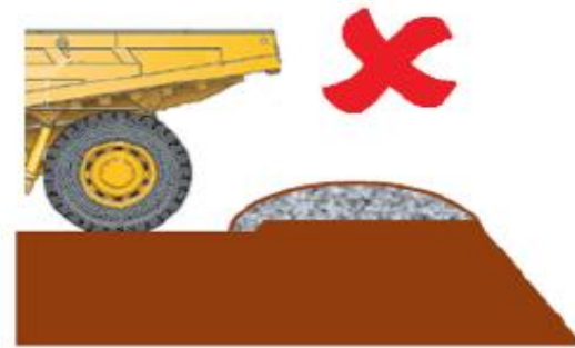
UNSUITABLE EDGE PROTECTION BERM PROFILE
